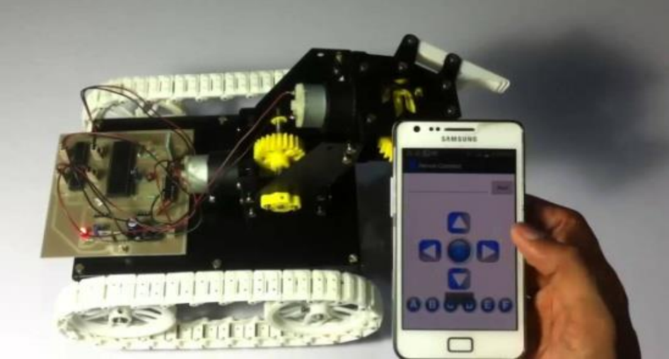
Touch Screen Based Remote Controller Robot With Wireless Camera.
