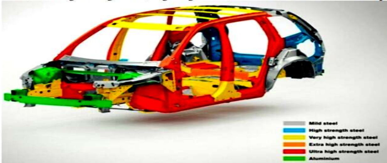
Figure 3. The materials used in new XC90 (Courtesy of Volvo Car Corporation)
