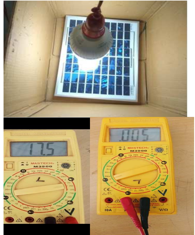
Figure 6. Solar panel with light source and without reflector arrangement and its measurements
