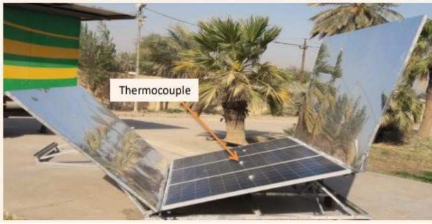
Figure 1. Schematic View of Solar panel with Light Reflector Arrangement panel with Light Reflector Arrangement
