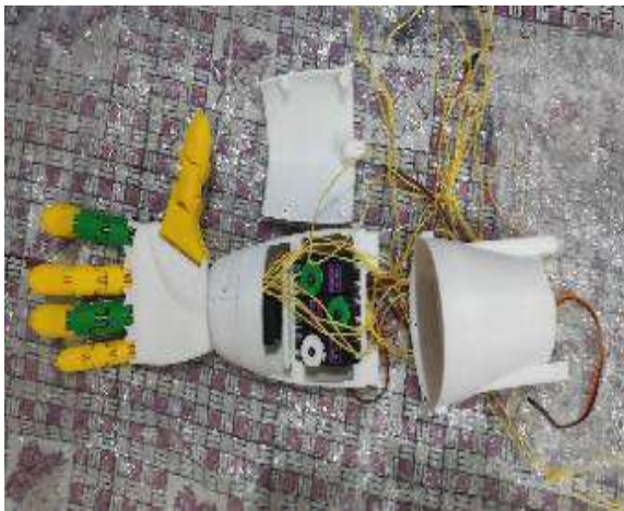
Fig.3. Fingers are controlled by tendons actuated through servo motors placed in the forearm
