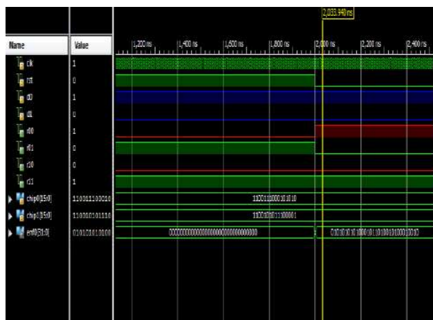
Fig. 4 Simulation result of 16-bit orthogonal gold code of CDMA system with two nodes
