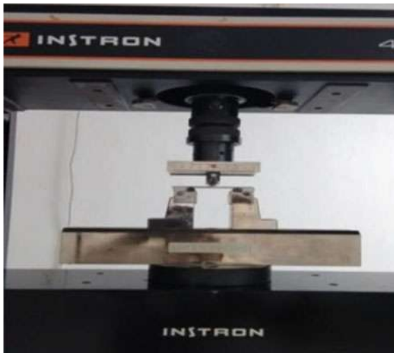
Fig. 10 Flexural test set-up
