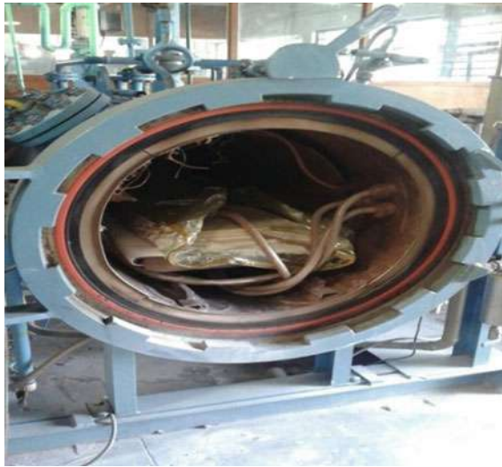
Fig. 4 Curing process using autoclave
