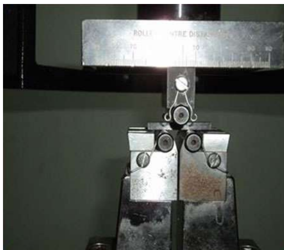
Fig. 14 Three-point bend test set-up
