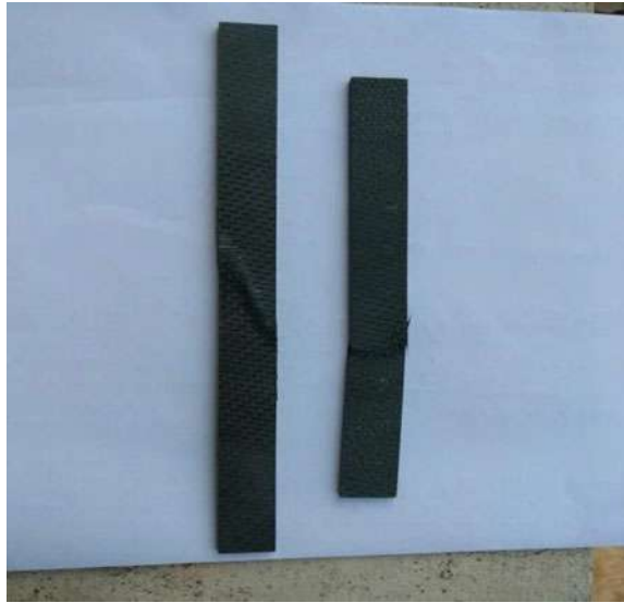
Fig. 7 Tensile failure modes
