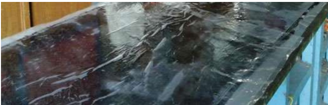
Fig. 2 Hybrid resin impregnated on carbon fabric
