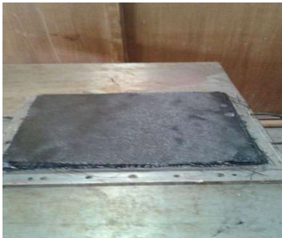
Fig. 3 Prepreg cut into 300 \times 300 mm size
