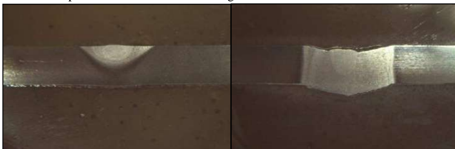
Fig 3. Macrostructure of weld (a) with Argon shielding gas (b) with Argon-Hydrogen shielding gas
