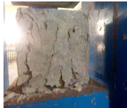
failure of cube
