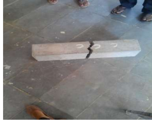
failure of beam
