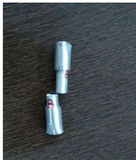
Fig. 3 Tensile test specimen after the test.
