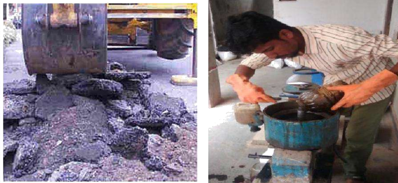
Fig. 1 Collection RAP material and bitumen extraction test on RAP
